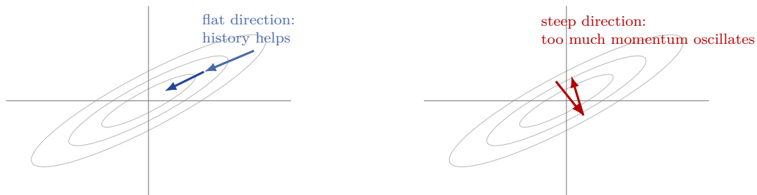
Figure 10.2: Momentum as a filter on directions. Left: along the valley successive steps agree and accumulate. Right: across the valley they alternate and cancel; with too large a \beta the alternation is amplified instead.
